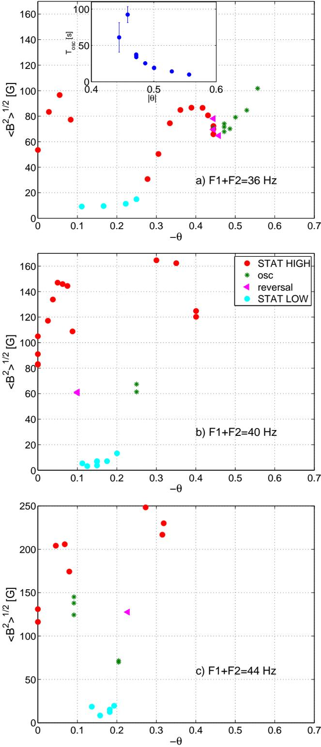
**Fig. 5.** (a) Transition plots as asymmetry ( $\theta$ ) is varied at fixed  $F$ . a)  $F_1 + F_2 = 36$  Hz. Color code as in (b). The inset shows the corresponding evolution of the period of oscillation in the oscillating/reversing regimes. (b)  $F_1 + F_2 = 40$  Hz. (c)  $F_1 + F_2 = 44$  Hz. Color code as in (b).
