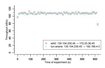
Fig. 6. Download using MPTCP and traffic control
