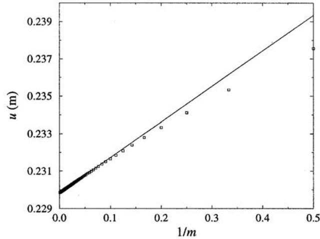
Figure 3. Displacement convergence versus the inverse number of right and left blocks for the element under a load  $P = E$  (16-element discretisation,  $L/l = 16$ ). The line is the linear regression with respect to equation 6. The elastic block properties are  $\nu = 0.3$ ,  $h/l = 10$ .
