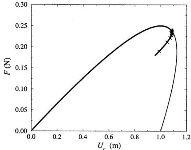
Figure 5. Global-Force displacement of a 32-element size,  $L/l = 32$ . Crosses correspond to the different damages profiles in Figure 6. The thin curve is the homogeneous behaviour. The elastic block properties are  $\nu = 0.3$ ,  $\bar{E} = 2$ ,  $h/l = 4$  m.
