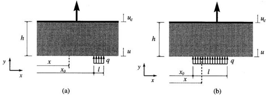
Figure 2. In the two schemes, just the elastic block is represented. On the left (a), displacement is measured *outside* the location of the distributed load. On the right (b), displacement is measured *inside* the location of the distributed load.
