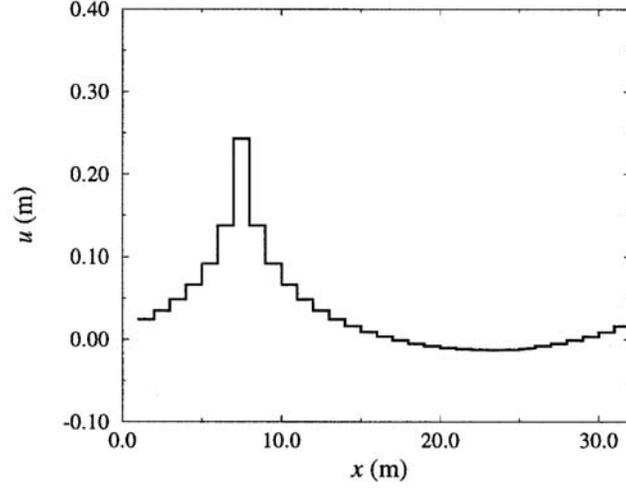
Figure 4. The deformation  $u$  of one block of width  $L/l = 32$  (32 elements) with periodic conditions, under a pressure applied on an unit length segment  $P = E$ . The elastic block properties are  $\nu = 0.3$ ,  $h/l = 10$ .
