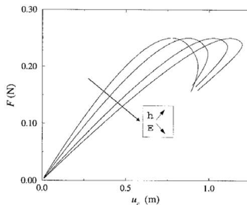
Figure 7. The force-displacement response of a system with 16 elements in the interface,  $L/l = 16$ . Initial stiffness decreases if  $h$  increases (for a fixed  $E$ ). Initial stiffness decreases if  $E$  decreases (for a fixed  $h$ ).
