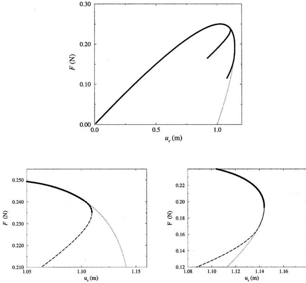
Figure 8. The force-displacement response of a system with 32 elements in the interface,  $L/l = 32$ . The elastic block Poisson ratio is 0.3. The two lower graphs are zooms on the bifurcation point. The left one corresponds to  $\tilde{E} = 4$  and  $h/l = 2$ . The right one corresponds to  $\tilde{E} = 14$  and  $h/l = 7$ . The stable states are represented by bold (continuous or dashed) lines, whereas the unstable states are represented by thin (continuous or dashed) lines.
