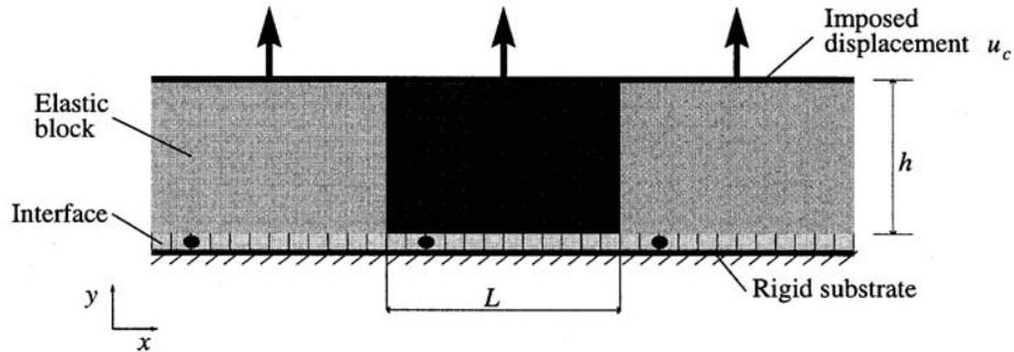
Figure 1. The interface, composed of  $n = 12$  elements, coupled in series with the elastic block. Three cells (blocks) are represented. The black circles in the interface are just plotted in order to better understand the periodic boundary conditions.
