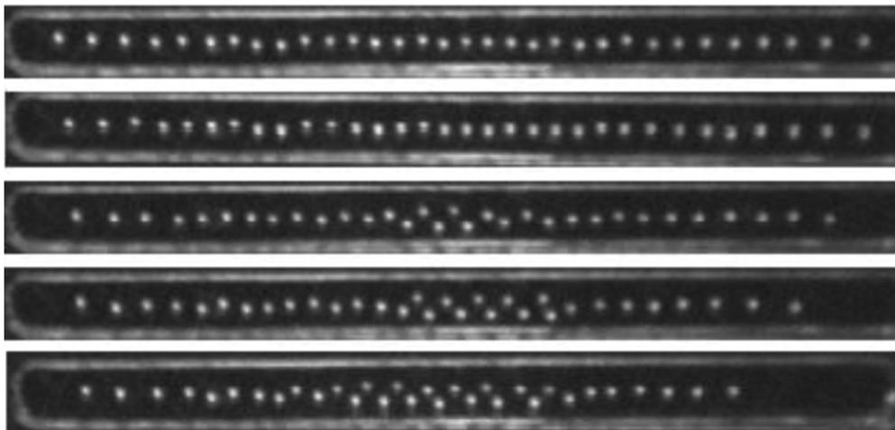
FIG. 2. Example of a zigzag transition in an experimental macroscopic system: 32 metallic beads in electrostatic interaction and confined in a finite-sized channel ( $L = 57$  mm) at an effective temperature  $T = 9 \times 10^{11}$  K adopt a zigzag configuration as the confinement decreases (from top to bottom).
