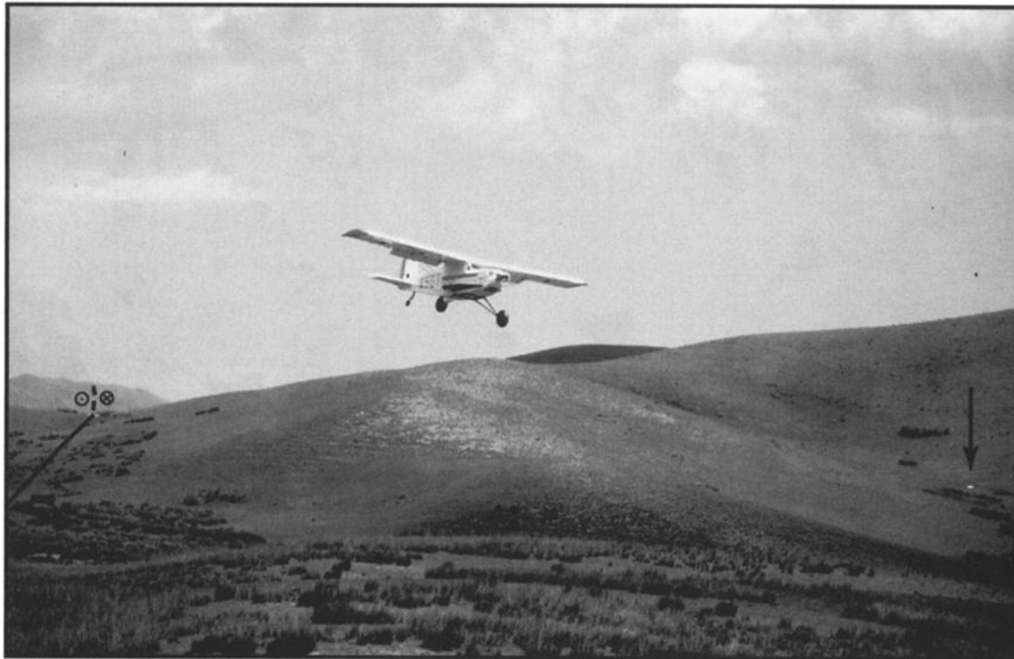
Figure 2. View of small remote-controlled airplane (3.3 m wingspan) flying above steppe along eastern swath (Figure 1a), before landing. Arrow points to one target used in stereopreparation of DEM (see discussion in text). Fault trace, on left side of photograph, is outlined.
