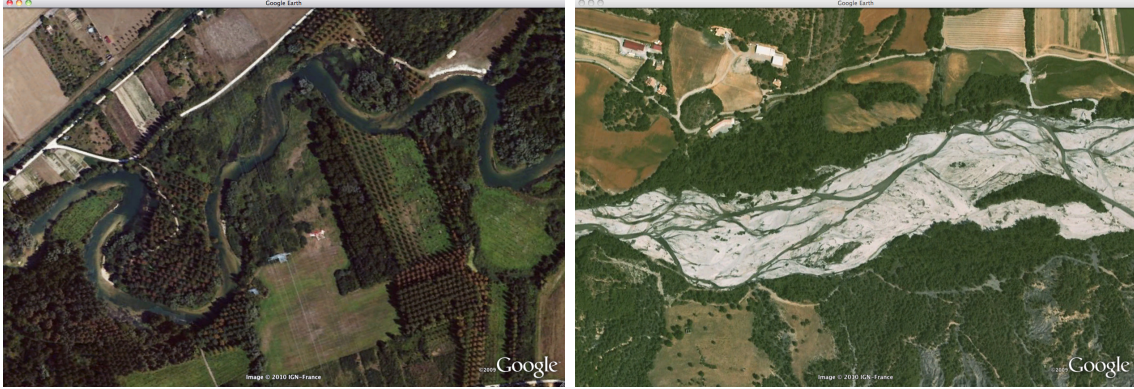
Figure 6: Typical examples of meandering and braided gravel bed streams. Meandering: Seine river near Méry-sur-Seine, France; braided: Bléone river in the French Alps near Dignes-les-Bains. The width of flow is 20-30 m in both cases. Images from Google earth.
