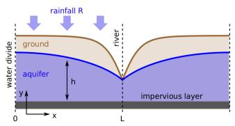
Figure 1 Schematics of an aquifer, and associated notations. The rainfall water fills the aquifer, which in turns flows into a stream. The porous rock is dissolved by groundwater, the concentration of which depends on the shape h(x) of the aquifer
