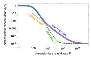
Figure 3 Theoretical concentration-discharge relationships for H=100 and  $c_r/c_s$ =10<sup>-5</sup>. The complete solution requires the numerical integration of equation (8), whereas the two asymptotic behaviors correspond to the analytic expressions (13) and (20)
