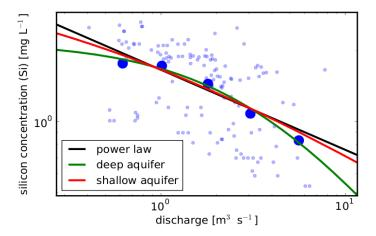
Figure 5 Concentration of Silicon as a function of discharge in the Ür ümqi River, China (small blue dots). All three models have two adjustable parameters. Power-law:  $c=1.7Q^{-0.34}$  (if c and Q are expressed in mgL<sup>-1</sup> and m³s<sup>-1</sup> respectively); deep aquifer:  $c_s$ =2.2 mgL<sup>-1</sup> and  $Q_c$ =3.3 m³s<sup>-1</sup>; shallow aquifer:  $c_s$ =5.1 mgL<sup>-1</sup> and  $Q_c$ =0.45 m³s<sup>-1</sup>. The large blue dots represent bin averaged data
