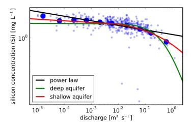
Figure 6 Concentration of Silicon as a function of discharge in a stream of the Mont Loz ère, France (small blue dots). All three models have two adjustable parameters. Power-law:  $c=1.1Q^{-0.05}$  (if c and Q are expressed in mgL<sup>-1</sup> and m³s<sup>-1</sup> respectively); deep aquifer:  $c_s=1.5$  mgL<sup>-1</sup> and  $Q_c=0.65$  m³s<sup>-1</sup>; shallow aquifer:  $c_s=1.7$  mgL<sup>-1</sup> and  $Q_c=2.2$  m³s<sup>-1</sup>. The large blue dots represent bin averaged data
