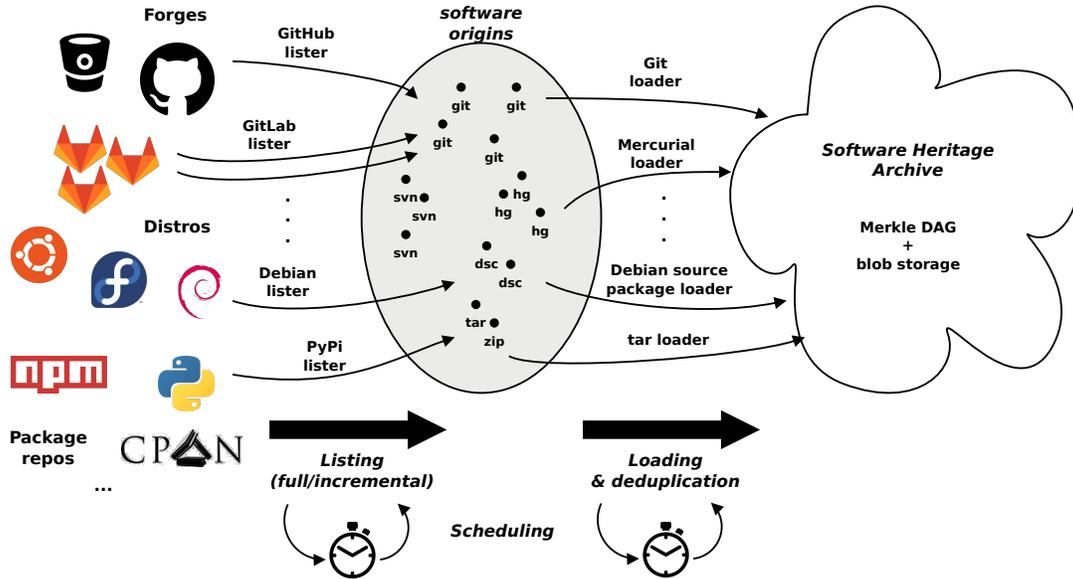
Figure 4: Ingestion data flow in Software Heritage
