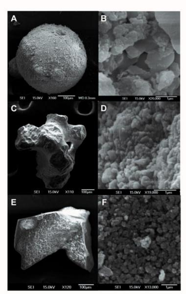
Scanning electron micrographs of HA/TCP (A-B), coral (C-D) and BG (E-F) granules at low (A-C-E) and high (B-D-F) magnification.
