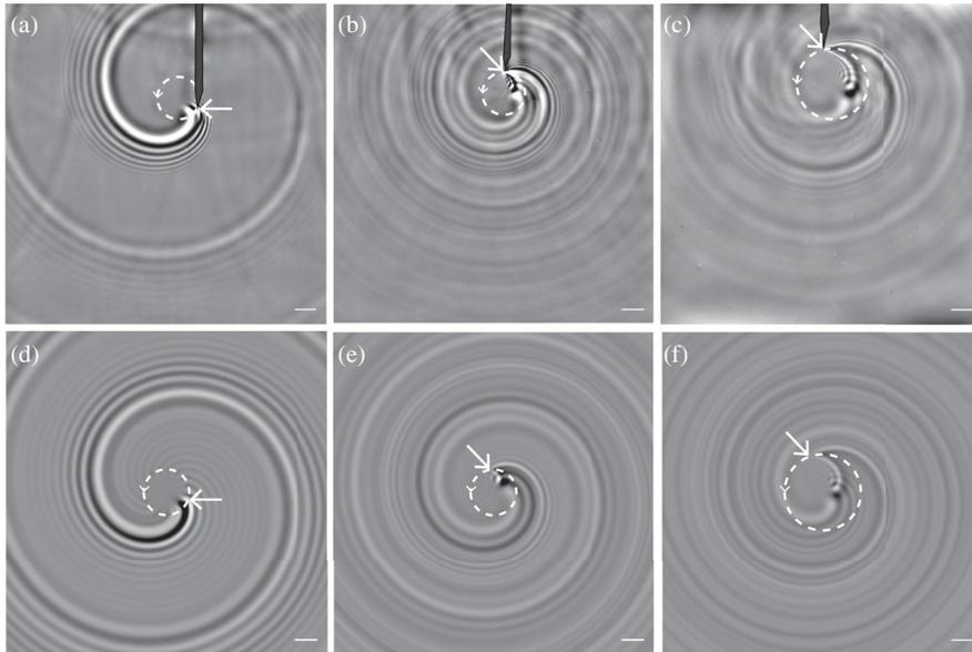
FIG. 3. (a)–(c) Experimental wave fields produced on the water surface by a pressure source moving on a circular path at  $Ma_{\min} = 1.2$ ,  $Ma_{\min} = 2$  and  $Ma_{\min} = 3.3$  respectively. (d)–(f) show corresponding wave fields computed from the hydrodynamic model. White oriented dashed circles depict the source trajectories while white arrows point at the current positions of the sources. 1.5 cm long white bars are superimposed on the fields for scale.
