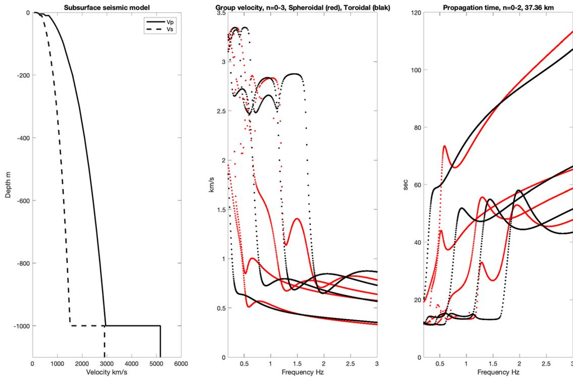
**Figure 3.** (left) Subsurface seismic model. (middle) Group velocities of the fundamental Rayleigh and Love waves and of the three first spheroidal (red) and toroidal (black) overtones. (right) Propagation time of the surface wave packet to a distance of 37.36 km, as a function of frequency up to 3 Hz. Model data is provided in Table S2.
