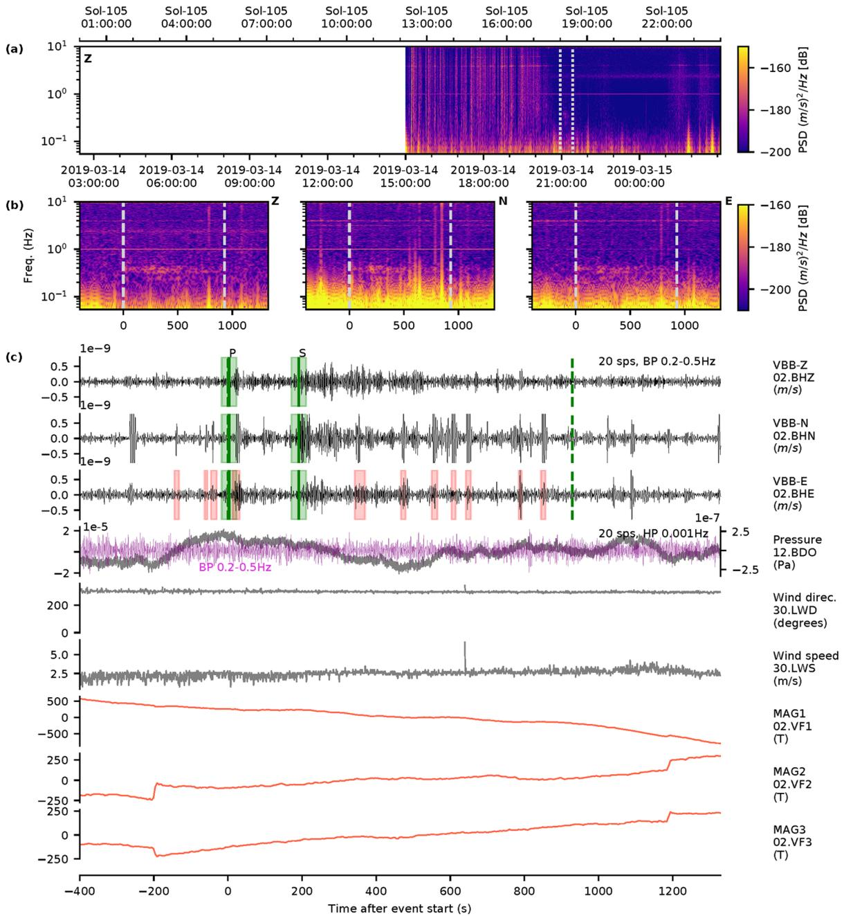
**Figure 6.** Summary of S0105a event, following Figure 5. During this event, there are multiple glitches (red shaded windows), most clearly visible in the E component, and no lander activity. MQS also identifies P and S phases (green solid vertical lines). Event energy is visible on all three components in both time series and spectrograms.
