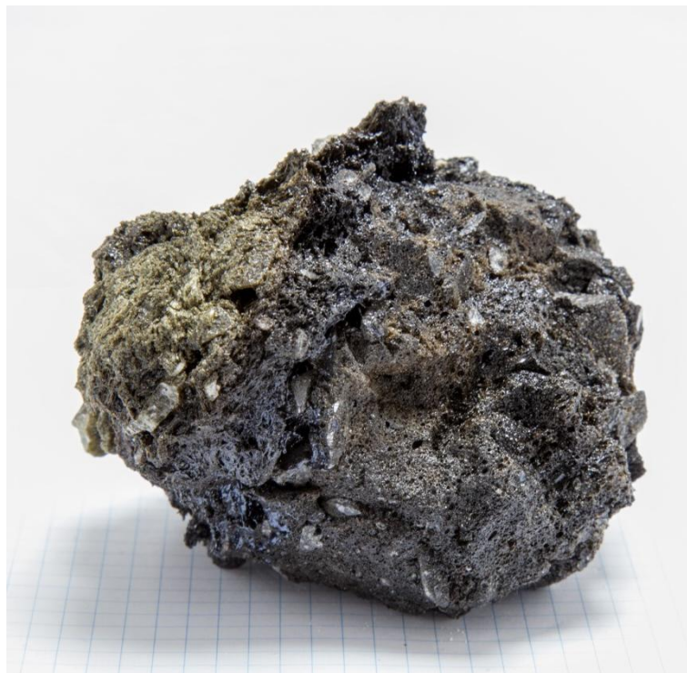
Figure 5 – Bomb sample from Erebus volcano with the surface covered by olive green and black glass with a metallic lustre, and anorthosite crystals. Image copyright: D.R. Neuville (square dimension=5mm).
