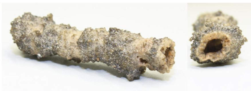
Figure 13 - Photographs of a fulgurite sample. The inner part is more smoothed and has a heterogeneous glassy material, whereas the outer portion is very irregular. Image copyright: M.R. Cicconi. Length of the specimen: ~5.5 cm.
