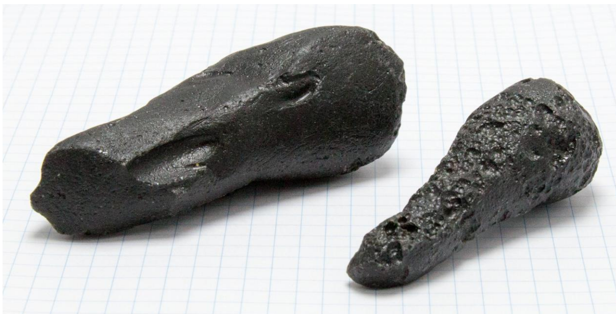
Figure 8 – Tektites specimens with the typical aerodynamic shapes and characteristic surface features. Image copyright: D.R. Neuville (square dimension=5mm)
