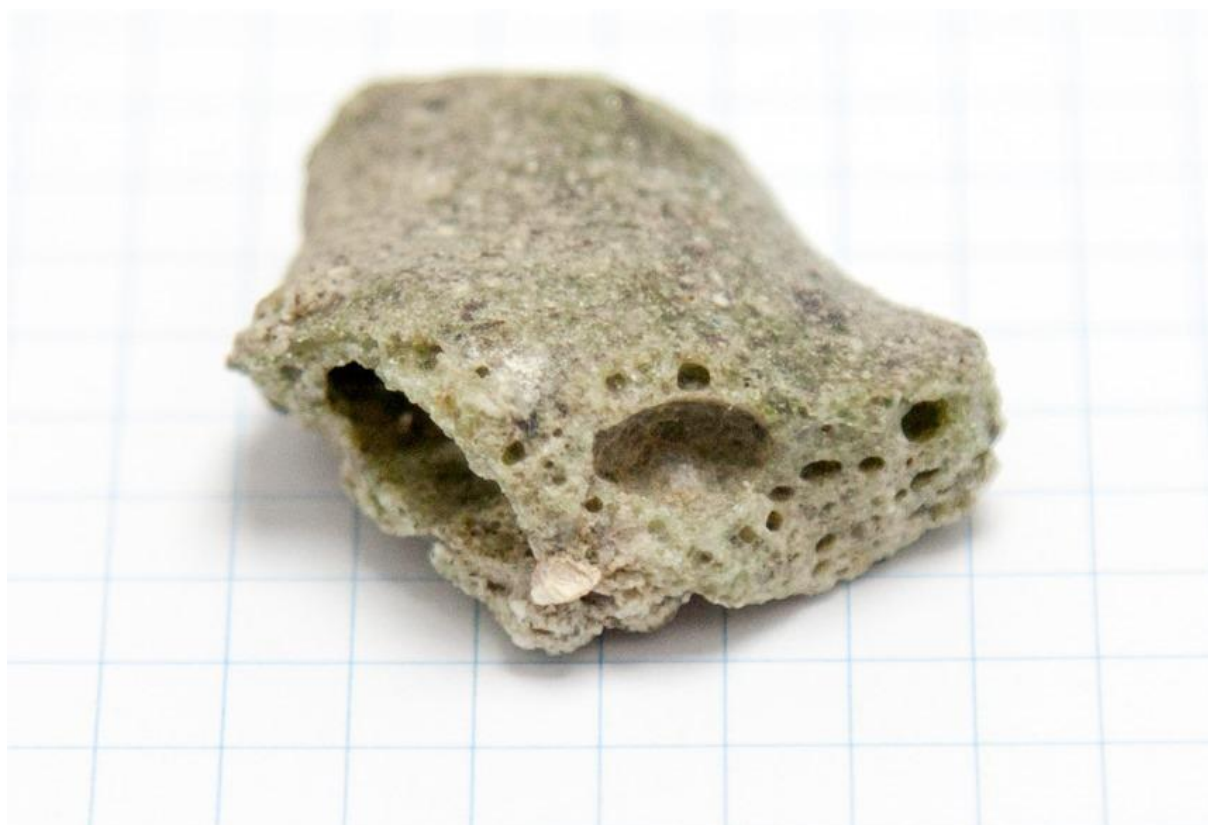
Figure 19 – Glass sample from Trinity site, Tularosa Basin, Alamogorgo (USA). This green trinitite fragment is glassy and vesiculated and is a product of the first atomic bomb blast on July 16, 1945. Image copyright: D.R. Neuville (square dimension=5mm).
