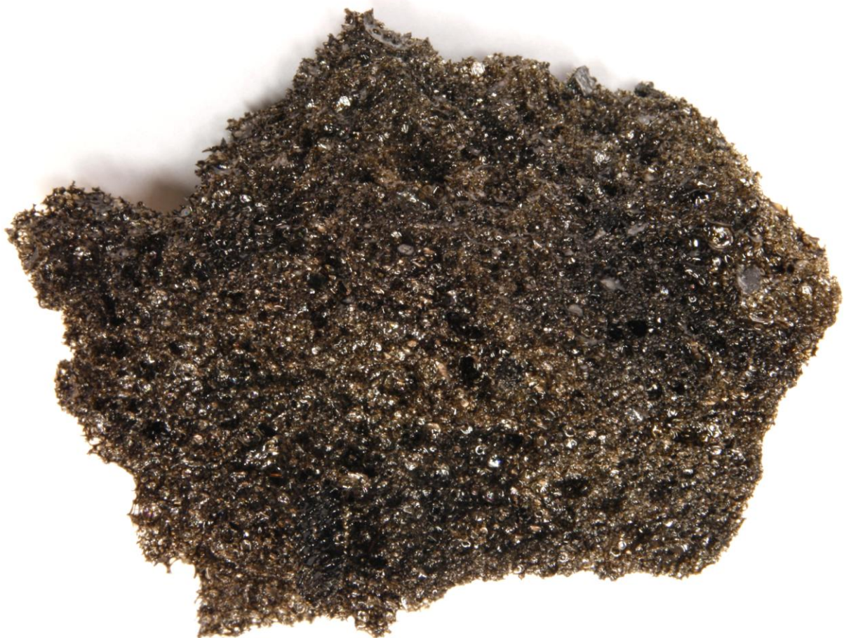
Figure 3 – Reticulite from Erebus volcano. This highly foamed sample is mainly composed of glass. Image copyright: D.R. Neuville (sample dimension 7x6x5cm).
