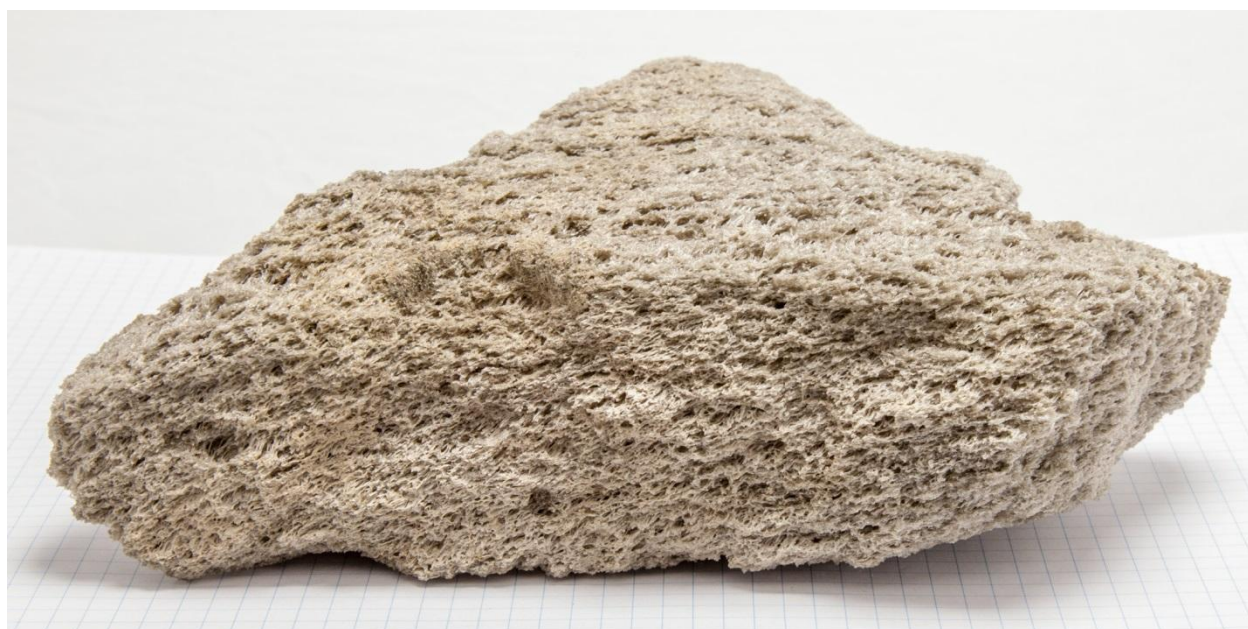
Figure 17 – Photograph of a pumice specimen from Glass Mountain (USA). The sample has the typical highly vesicular irregular texture. Image copyright: D.R. Neuville (square dimension=5mm).
