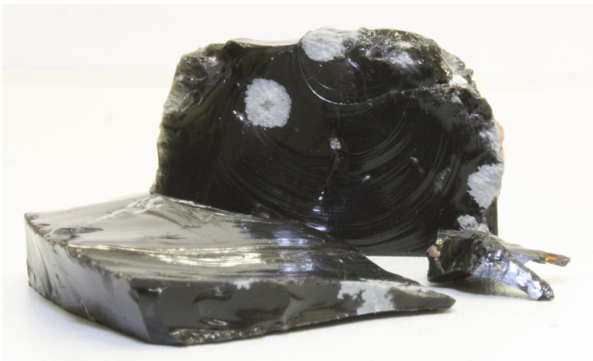
Figure 18 - Photograph of spherulitic obsidians (length ~ 4 cm; unknown locality). Spherulites are distributed homogeneously all over the samples with size ranging from 3.0 to 8.0 mm. Image copyright: M.R. Cicconi
