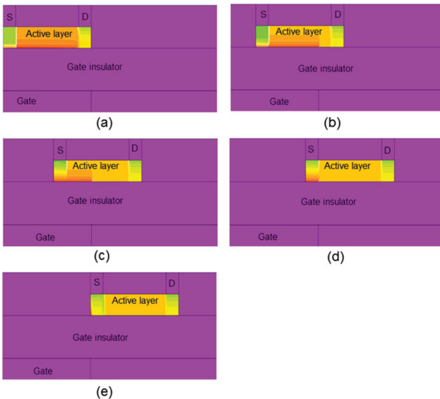
Figure 4. Hole concentration distribution in organic TFTs for gate voltage = drain voltage = -40 V; color-coded hole concentration values; represented by a continuous distribution from a maximum of 10^{19} to a minimum of 0 from red to purple, respectively. L_M is varied (a) 0 \mu\text{m} , (b) 20 \mu\text{m} , (c) 40 \mu\text{m} , (d) 60 \mu\text{m} , and (e) 70 \mu\text{m} .
