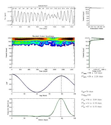
Fig. 2. Analysis of the rotation of KIC 6307037. *Left: from top to bot-tom: Kepler* light curve, WPS, autocorrelation function, and composite spectrum. *Right: from top to bottom:* power spectrum, global WPS, and results of the analysis.
