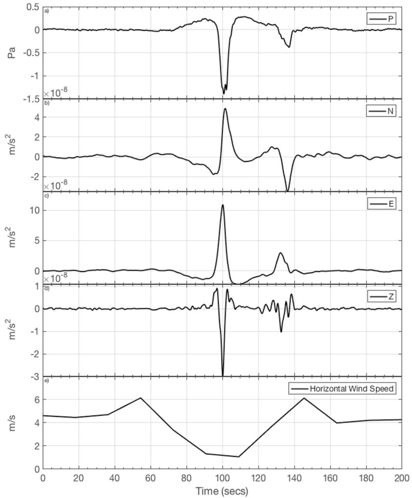
**Figure 5.** The pressure variation (P) measured by the barometer, the acceleration measured by the VBB sensor (N, E, and Z), and the horizontal wind speed measured by TWINS during 200 s around a convective vortex encounter. This event occurred on Sol 133 (April 12, 2019) at 9:51 UTC (12:34 LMST). In addition to the data processing described in Section 2, the data have been filtered in the (0.02–0.3 Hz) frequency band.
