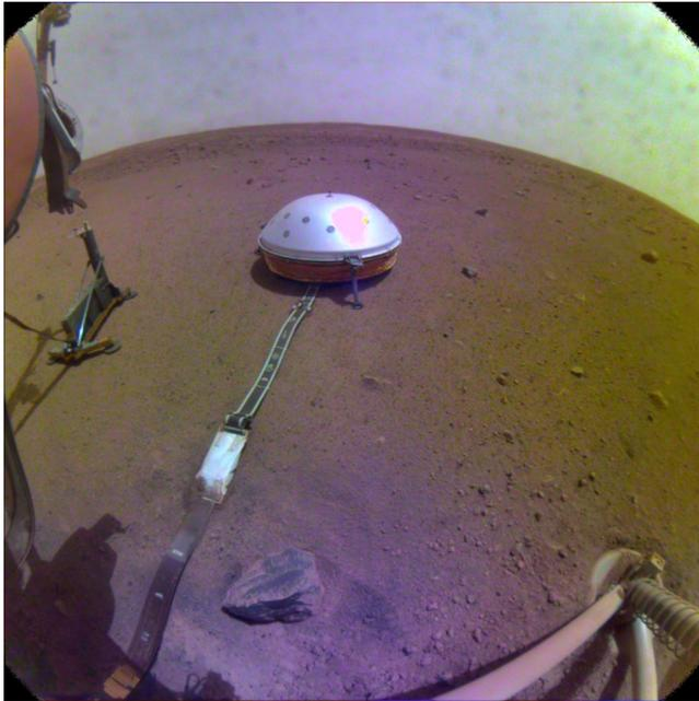
**Figure 2.** SEIS and the “Wind and Thermal Shield” deployed on the surface of Mars. This image, taken by InSight’s context camera, also shows the electrical cable linking SEIS to the lander, the Heat Flow, and Physical Properties Package instrument to the left of SEIS, and one of the lander feet in the bottom right of the image. Image courtesy of NASA/JPL/Justin Maki.
