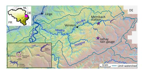
**Figure 1.** (a) The Vesdre watershed (702 km<sup>2</sup>) and (b) enlarged view around the Membach station, with the Gileppe and Eupen reservoirs, the Béthane hamlet and the Jalhay rain gauge. The water mass in the areas circled in black contributes 90% (solid line) and 95% (dotted line) of the gravity signal as monitored by the gravimeter. The purple square represents the footprint of the weather radar. Maps from Walloon Geoportal https://geoportail.wallonie.be/walonmap.
