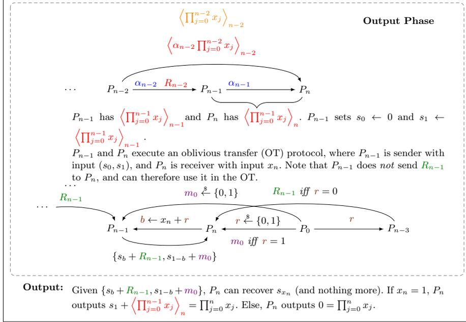
Fig. 4: Output phase of the 1-private protocol for the  $(n+1)$ -AND functionality. Each party  $P_i$  has an input bit  $x_i$ .  $P_n$  receives the output  $\prod_{j=1}^n x_j$ . The protocol uses six random bits in total  $(\alpha_0, R_1, \langle x_0 \rangle_0, \langle \alpha_0 x_0 \rangle_0, m_0, r)$ , which are all generated by the single random source  $P_0$ . The color of a value indicates which of the six random bits masks it additively. All operations are over  $\mathbb{F}_2$ .
