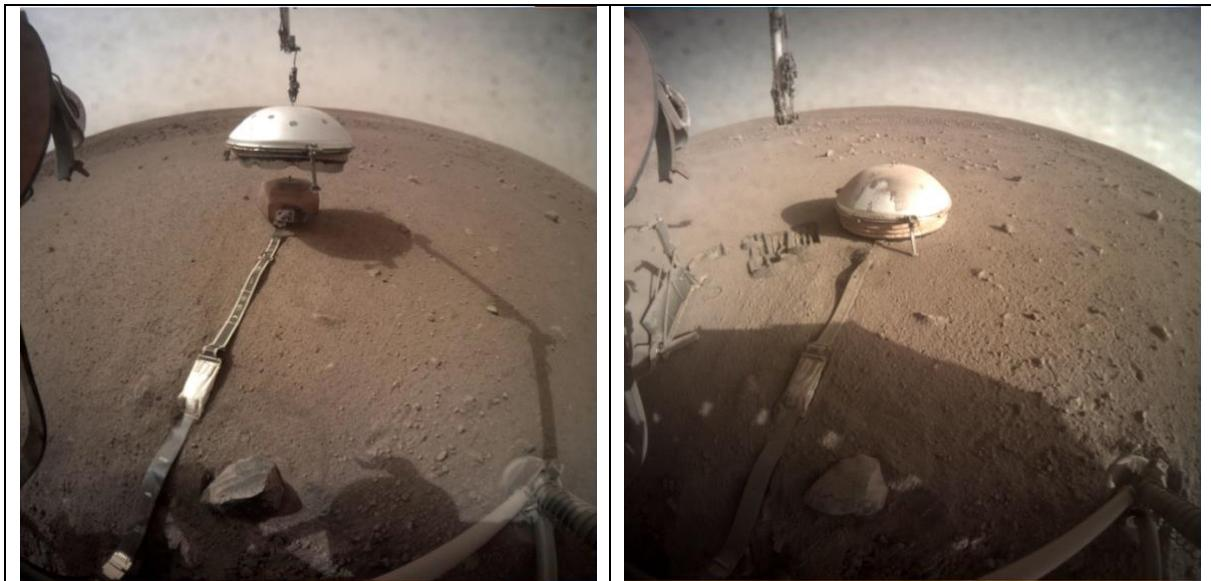
Figure 1: A) The Sensor assembly of SEIS on the ground just prior the deployment of the Wind and Thermal Shield (WTS), on February 2, 2019. B) Picture taken on September 27, 2021 showing the fully installed WTS two and a half years later. These two images were taken on sol 66 and sol 1008 since InSight landing, respectively.
