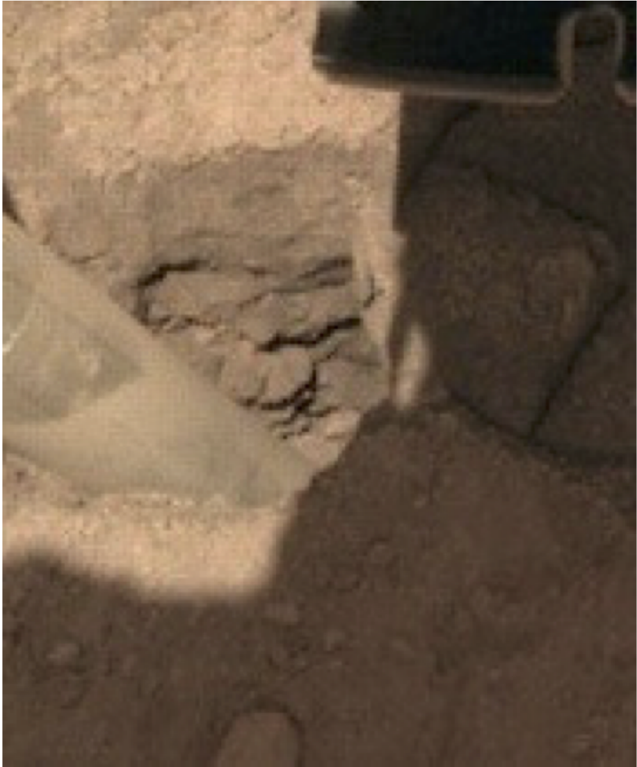
Fig. 10 Image of the hole created by the HP 3 mole showing the almost vertical southerly wall of the pit and resistant layers in it. These layers have steep edges and overhangs indicating cohesion in the soil. Small rocks appear cemented in a fine-grained matrix, similar to the pits beneath the lander. Mole is in the foreground angled \sim 15^\circ towards the right
