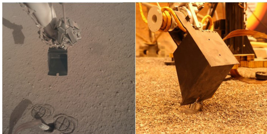
Fig. 4 The IDA scoop. In the left image, the scoop is shown above the HP 3 mole in this IDC image. The front blade is visible. The grapple is seen stowed to the side of the IDA forearm. In the right image, the scoop in the Earth-based testbed is shown in an “inclined push” configuration on the testbed mole back cap. The dull blade on the outside back of the scoop is visible
