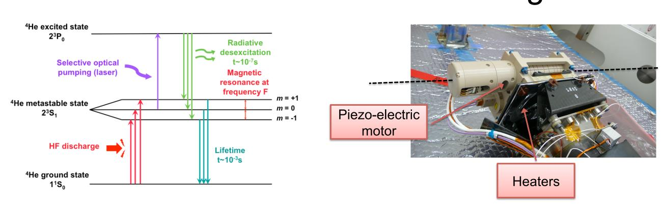
• The core of the ASM instrument is a **magnetic field to frequency** converter based on atomic spectroscopy of the <sup>4</sup>He in its metastable level 2<sup>3</sup>S<sub>1</sub>. It exploits the Zeeman effect, with the signal being amplified by optical pumping. The magnetic field modulus B<sub>0</sub> is directly proportional to the magnetometer's resonance frequency F:
