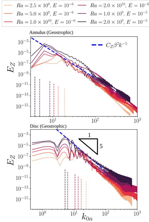
**Fig. 9.** Zonal spectra of the geostrophic velocity computed on the annulus (top panel) and on the disc (bottom panel). The theoretical prediction of the zonal spectra from Eq. (10b) corresponds to the dashed blue line using  $C_Z = 0.5$ . Vertical dashed segments are Rhines wavenumbers  $k_{Rh}$  from Eq. (20) and for each simulation. (For interpretation of the references to colour in this figure legend, the reader is referred to the web version of this article.)
