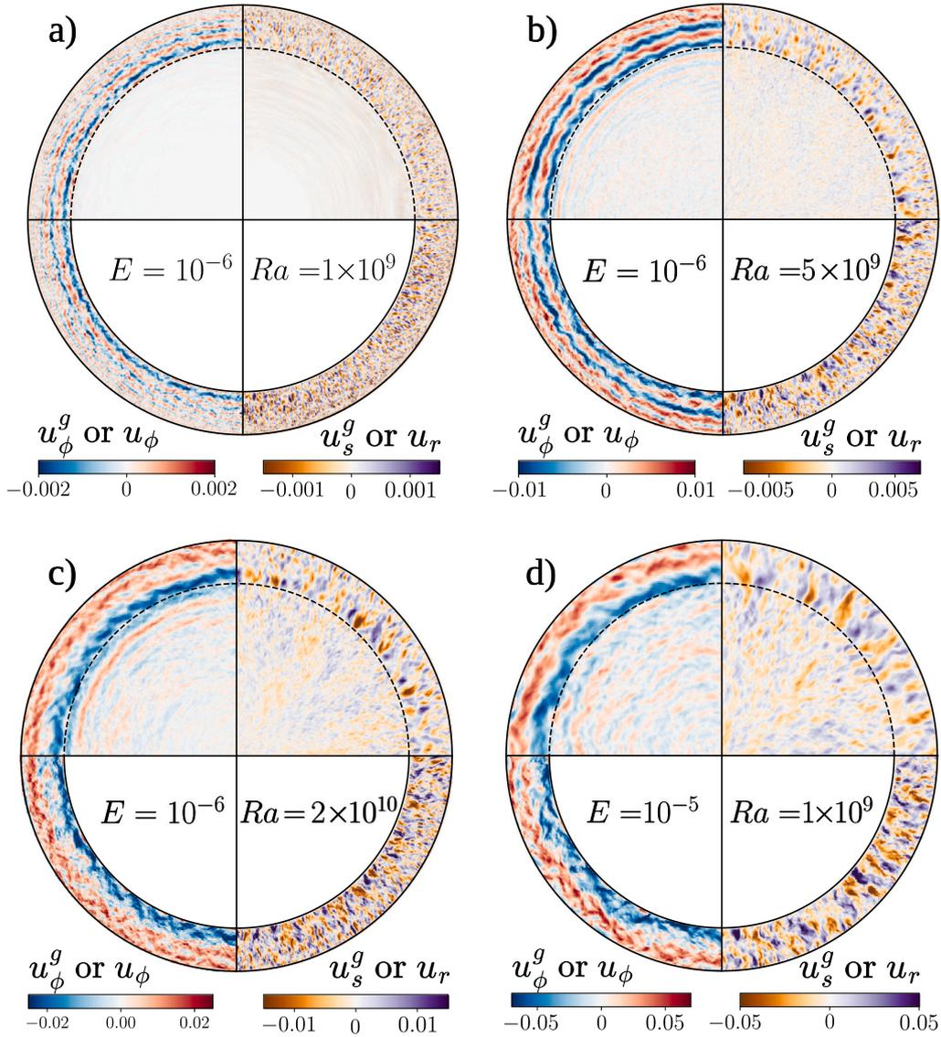
Fig. 6. Snapshots of different flow components for the four simulations shown in Figs. 4 and 5. For each panel, the upper half corresponds to the geostrophic flow components with  $u_\phi^g$  on the left and  $u_s^g$  on the right, while the bottom half corresponds to the flow in the equatorial plane with  $u_\phi(\theta = \pi/2)$  on the left and  $u_r(\theta = \pi/2)$  on the right. The dashed arcs in the upper halves mark the location of the tangent cylinder.
