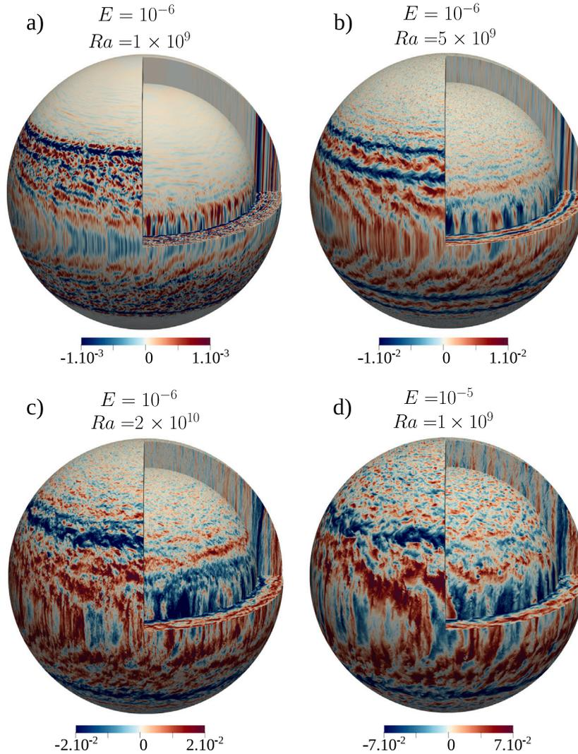
**Fig. 4.** Instantaneous zonal velocity maps in units of Rossby number, at  $r = 4.98$  for the outermost spherical surface and  $r = 4.05$  for the innermost one. The horizontal cut corresponds to the equatorial plane. Panels a–d correspond to simulations 1, 5, 7 and 15 in Table 1.
