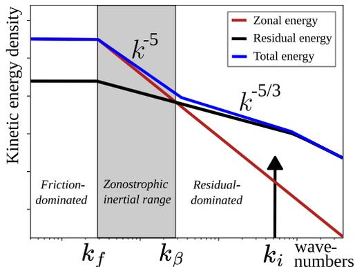
Fig. 2. Theoretical kinetic energy distribution as a function of wavenumber  $k$  in zonal and residual energy, after Galperin et al. (2010) and Cabanes et al. (2020).
