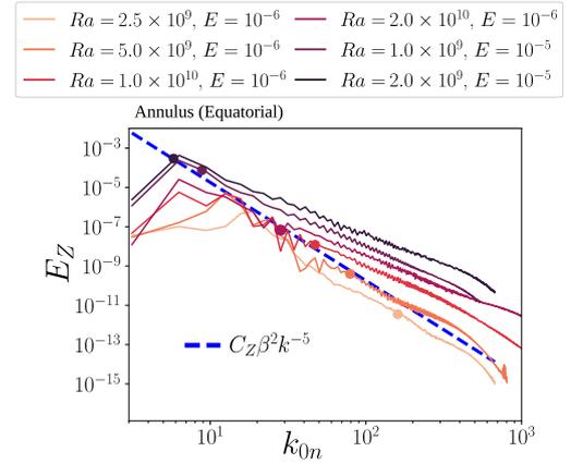
**Fig. 10.** Zonal spectra of the equatorial velocity computed on the annulus. The theoretical prediction of the zonal spectra from Eq. (10b) corresponds to the dashed blue line using  $C_Z = 0.5$ . Dots are Rossby scales  $k_{Ro}$  from Eq. (21). (For interpretation of the references to colour in this figure legend, the reader is referred to the web version of this article.)
